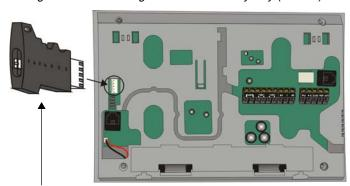
Jumper ON: Read from and/or write to memory key
